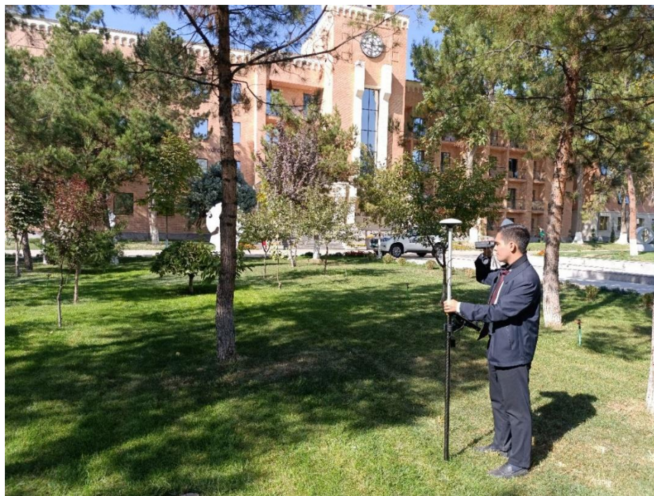
Figure 4. The process of determining tree coordinates using GNSS (Global Navigation Satellite System) technology in the field .
