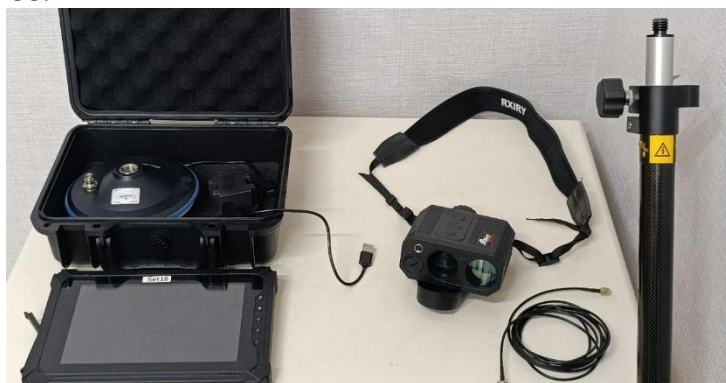
Figure 1. A set of field measurement equipment using GNSS (Global Navigation Satellite System) technologies.
